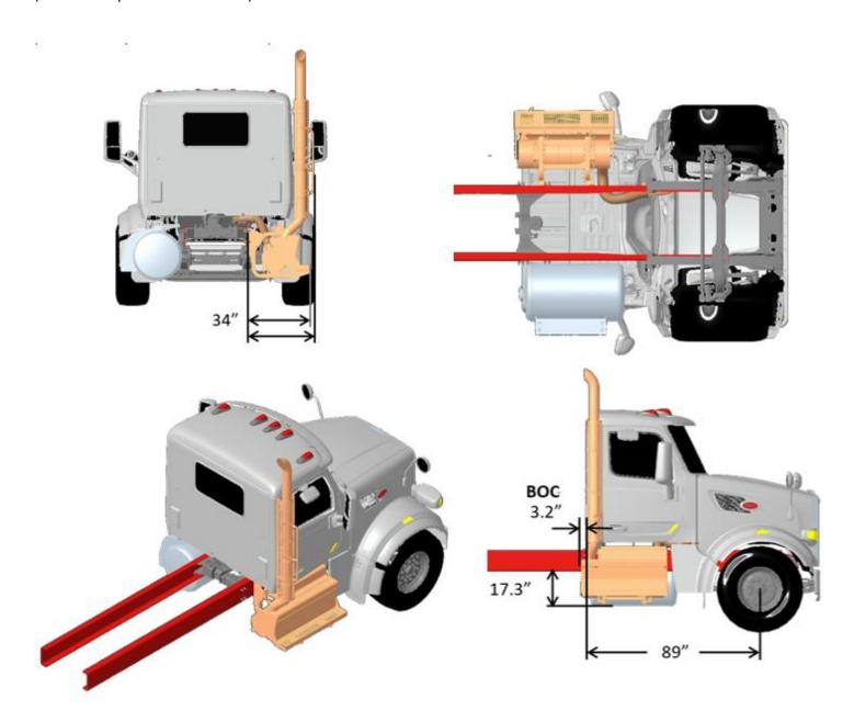
FIGURE 11-22: Model 567-121 SFFA RH Side of Cab Exhaust
