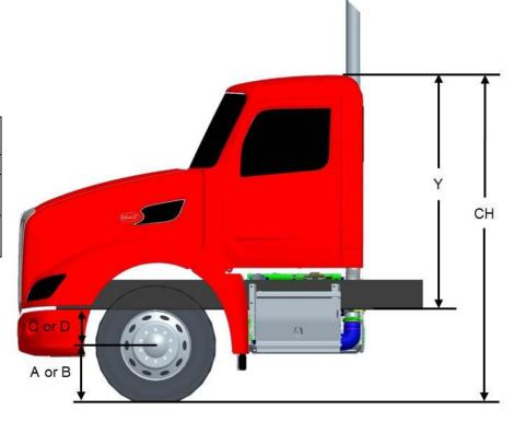
FIGURE 3-30. Overall Cab Height Calculations
