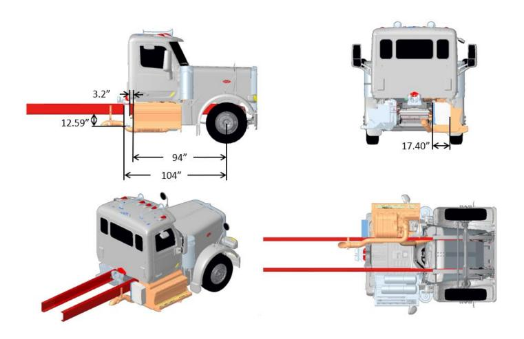
FIGURE 3-94. Exhaust Single RH Horizontal DPF/SCR RH Under Cab, Compact Twin
