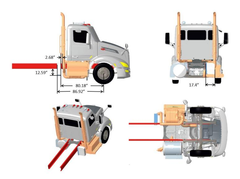
FIGURE 3-120. Exhaust Dual Back of Cab, LH BOC Stack Aesthetic Only, DPF/SCR RH Under Cab, Compact Twin
