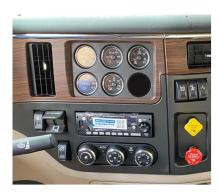
FIGURE 11-4: Dash Panel ready for F/O Fuel Pressure Gauge
