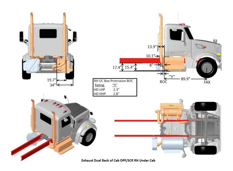
FIGURE 3-70. Exhaust Dual Back of Cab DPF/SCR RH Under Cab
