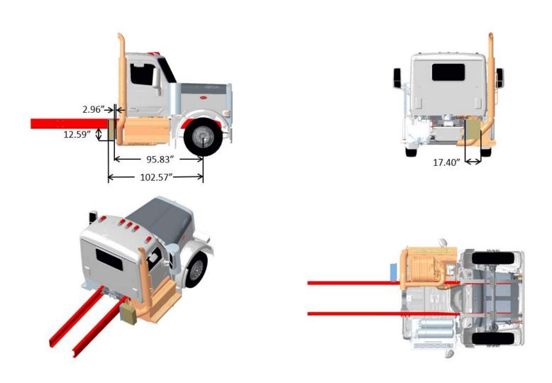
FIGURE 3-88. Exhaust Single RH Side of Cab DPF/SCR RH Under Cab, Compact Twin
