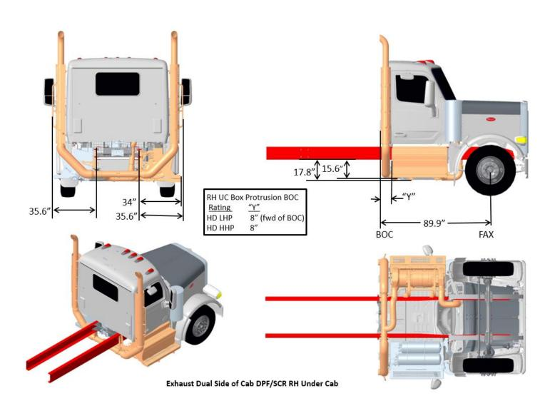
FIGURE 3-37. Exhaust Dual Side of Cab DPF/SCR RH Under Cab (functioning)
