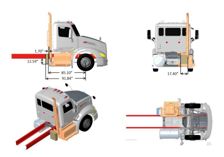
FIGURE 3-122. Exhaust Single RH Back of Cab DPF/SCR RH Under Cab, Compact Twin
