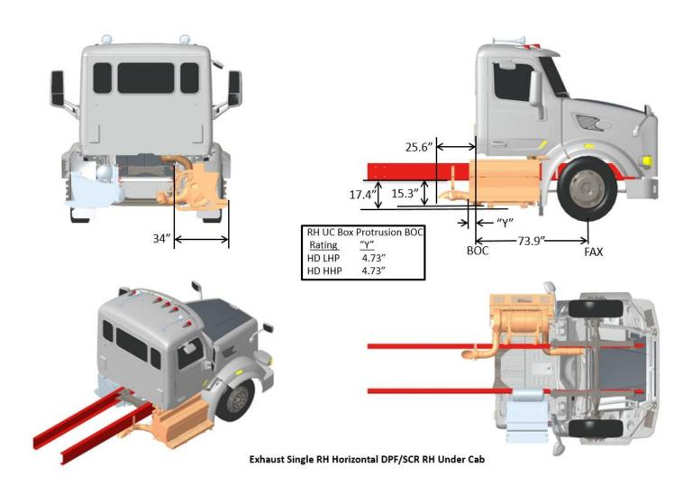
FIGURE 3-61. Exhaust Single RH Horizontal DPF/SCR RH Under Cab
