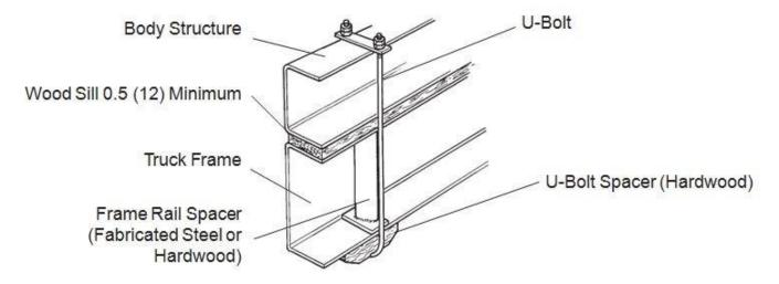
FIGURE 4-9. Acceptable U-Bolt Mounting with Wood and Fabricated Spacers
