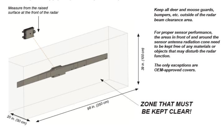
NOTE: Drawing is representative only and not to scale. Dimensions are accurate.
