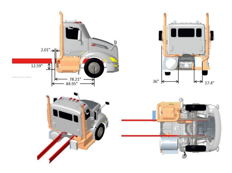
FIGURE 3-121. Exhaust Dual Side of Cab, LH SOC Stack Aesthetic Only, DPF/SCR RH Under Cab, Compact Twin
