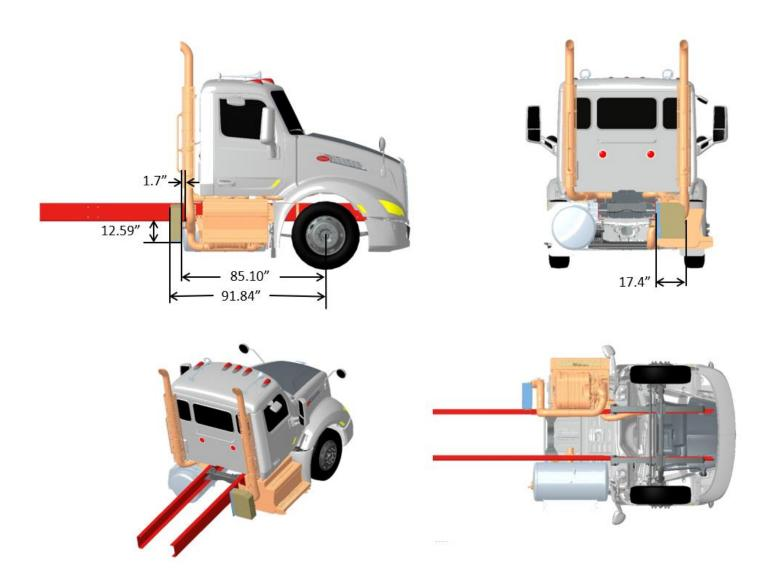
FIGURE 3-125. Exhaust Dual Back of Cab, LH BOC Stack Aesthetic Only, DPF/SCR RH Under Cab, Compact Twin
