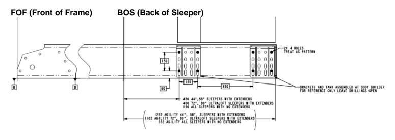
FIGURE 11-15: Back of Cab System Drilling (Agility)
