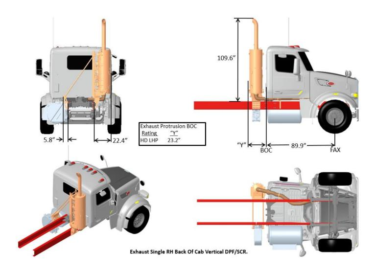
FIGURE 3-72. Exhaust Single RH BOC Vertical DPF/SCR
