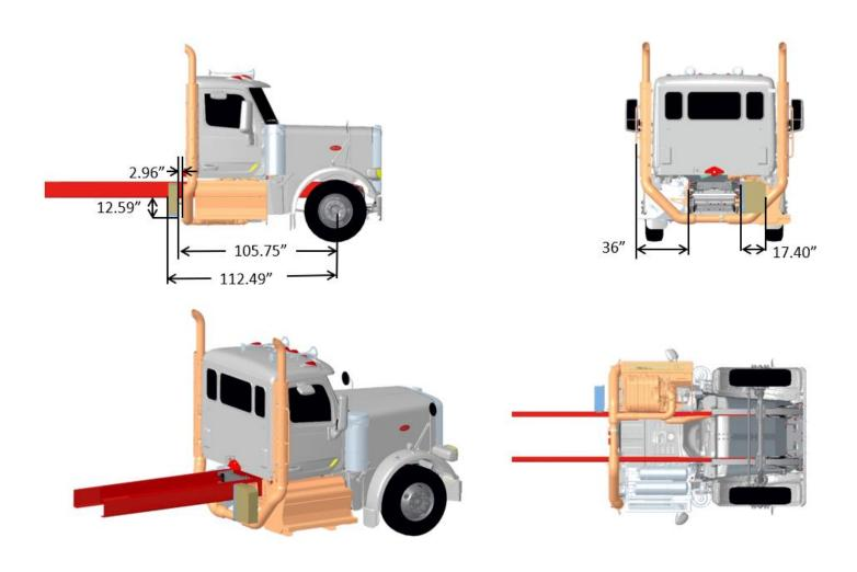
FIGURE 3-95. Exhaust Dual Side of Cab DPF/SCR RH Under Cab (Functioning), Compact Twin
