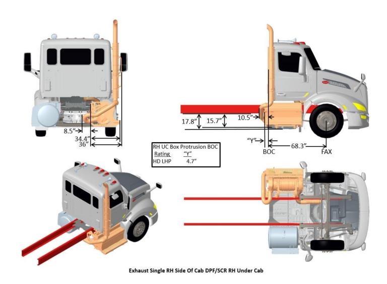
FIGURE 3-74. Exhaust Single RH Side of Cab DPF/SCR RH Under Cab
