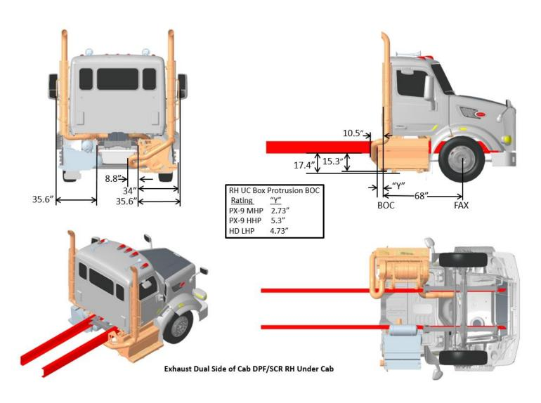
FIGURE 3-49. Exhaust Dual SOC DPF/SCR RH Under Cab
