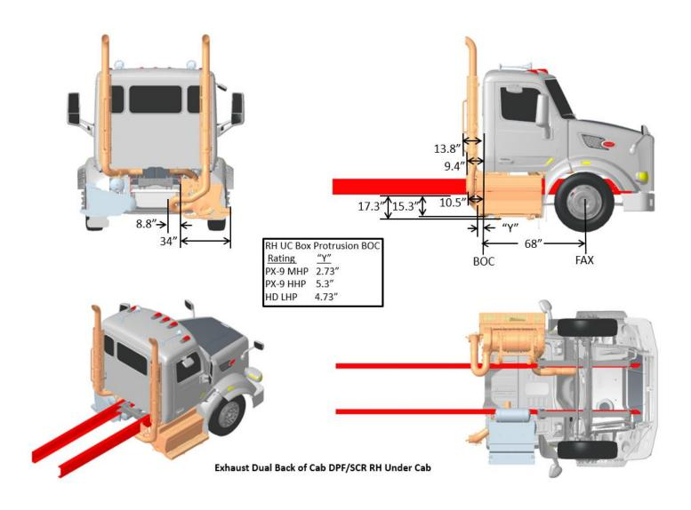
FIGURE 3-50. Exhaust Dual BOC DPF/SCR RH Under Cab
