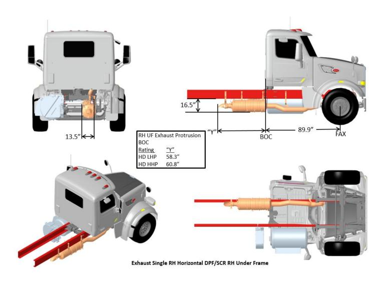
FIGURE 3-69. Exhaust Single RH Horizontal DPF/SCR RH Under Frame
