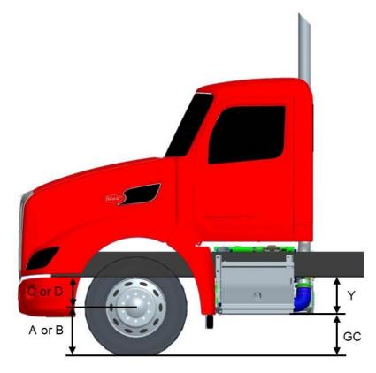
FIGURE 3-29. Ground Clearance Calculations
