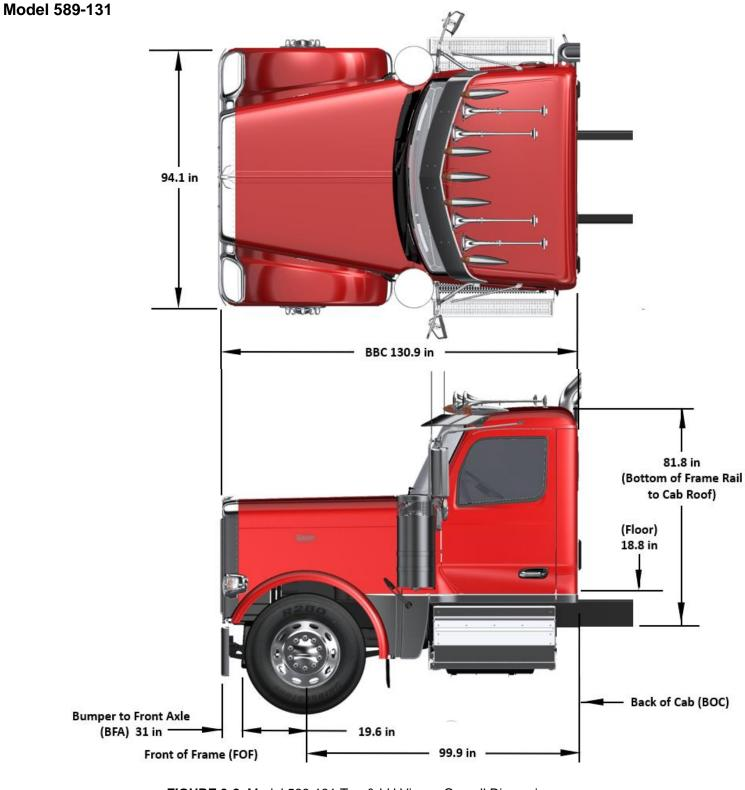
FIGURE 3-2. Model 589-131 Top & LH View – Overall Dimensions
