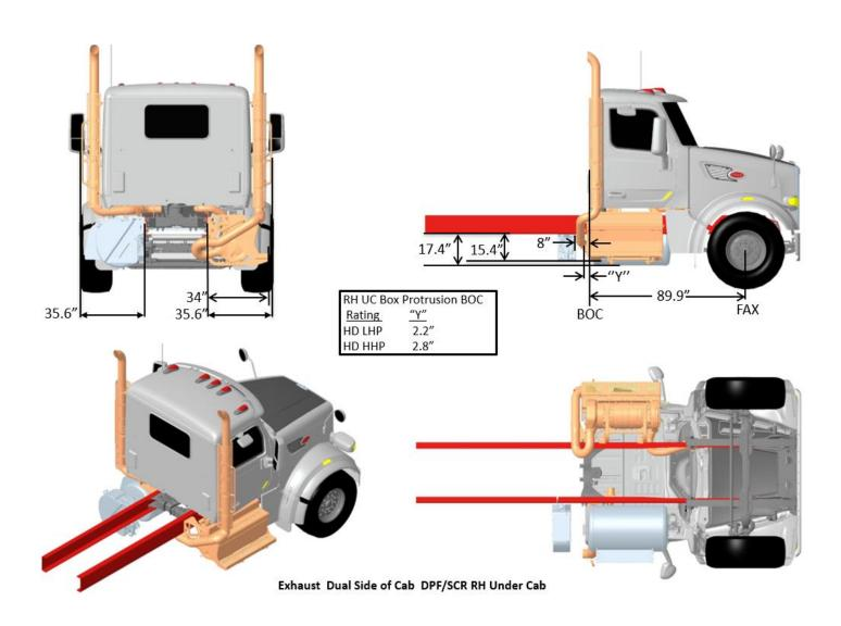
FIGURE 3-71. Exhaust Dual SOC DPF/SCR RH Under Cab
