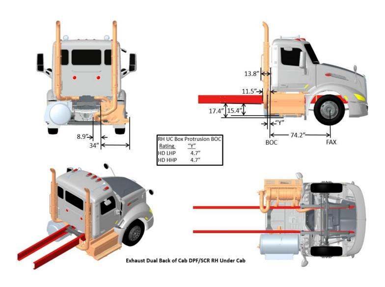
FIGURE 3-85. Exhaust Dual Back of Cab RH DPF/SCR RH Under Cab
