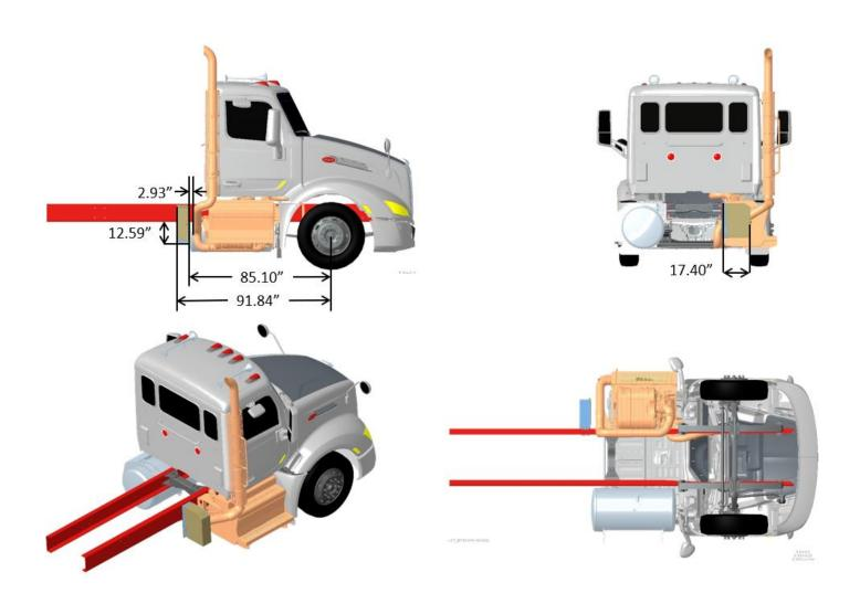
FIGURE 3-123. Exhaust Single RH Side of Cab DPF/SCR RH Under Cab, Compact Twin
