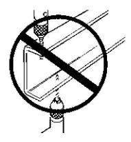
FIGURE 4-8. Frame Rail Flange Drilling Prohibited
