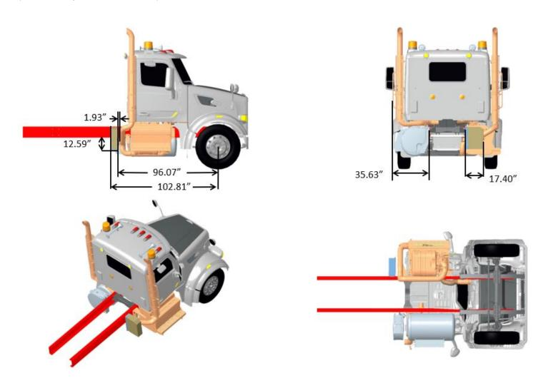
FIGURE 3-105. Exhaust Dual Side of Cab, LH SOC Stack Aesthetic Only, DPF/SCR RH Under Cab, Compact Twin
