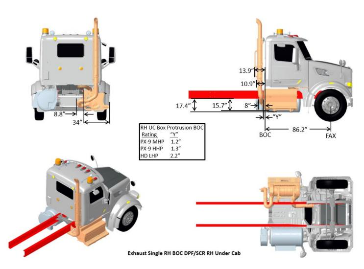
FIGURE 3-52. Exhaust Single RH Back of Cab DPF/SCR RH Under Cab
