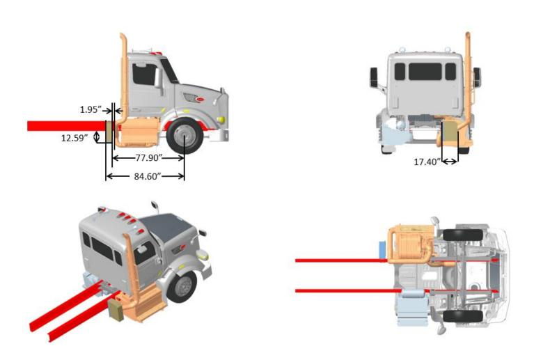
FIGURE 3-98. Exhaust Single RH Side of Cab DPF/SCR RH Under Cab, Compact Twin
