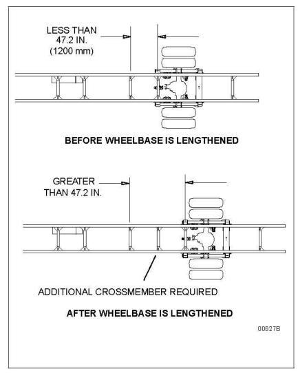
FIGURE 5-2. Crossmember Spacing Requirements
