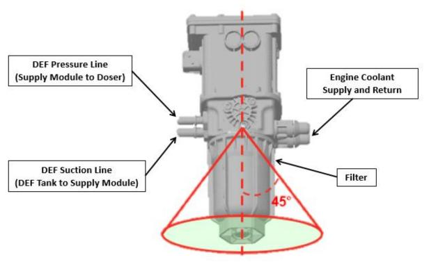
FIGURE 9-4. Supply Module Mounting Angle Limits
