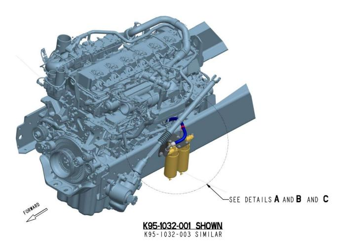
FIGURE 11-6: Fuel Routing and Fuel Filter Location
