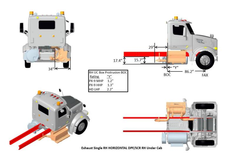
FIGURE 3-54. Exhaust Single RH Horizontal DPF/SCR RH Under Cab
