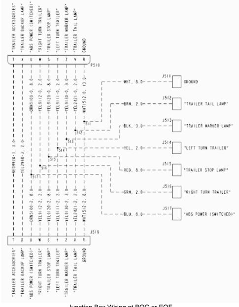
Junction Box Wiring at BOC or EOF
