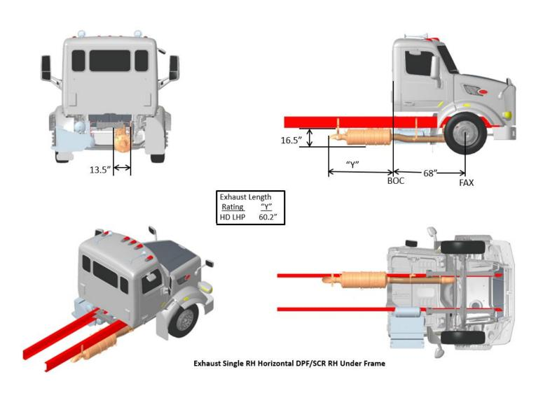
FIGURE 3-48. Exhaust Single RH Horizontal DPF/SCR RH Under Frame
