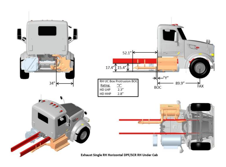
FIGURE 3-68. Exhaust Single RH Horizontal DPF/SCR RH Under Cab
