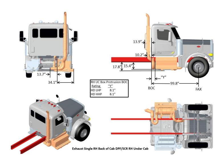
FIGURE 3-39. Exhaust Single RH Back of Cab DPF/SCR RH Under Cab
