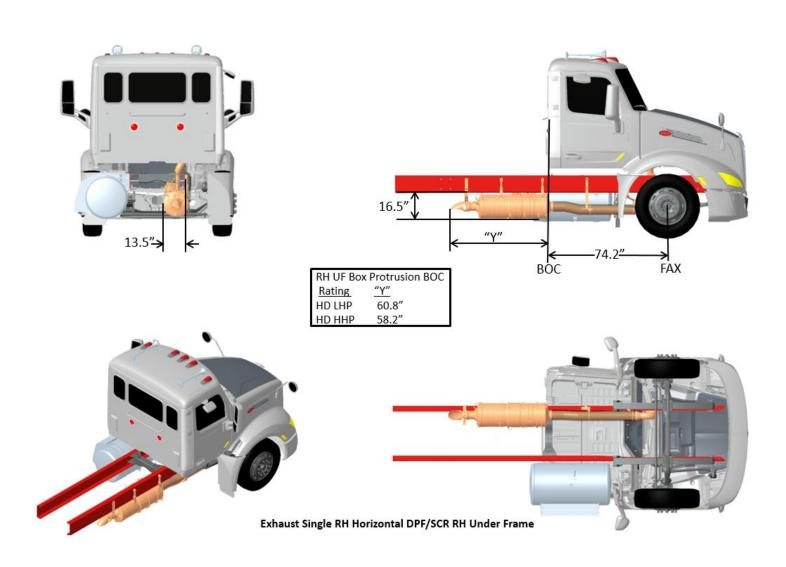
FIGURE 3-83. Exhaust Single RH Horizontal DPF/SCR RH Under Frame
