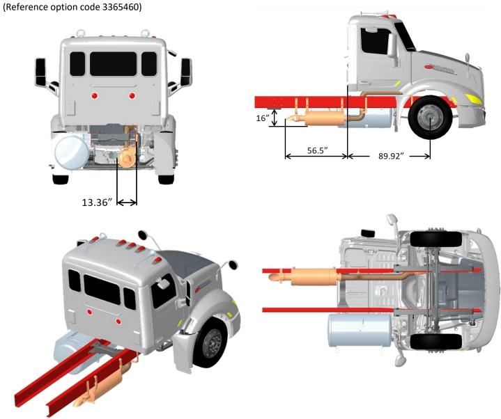
FIGURE 11-18: Model 579-124 RH Horizontal Underframe Exhaust
