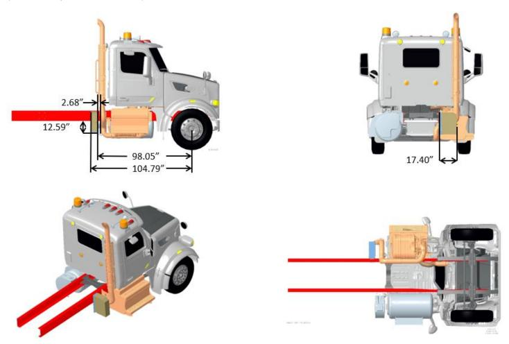
FIGURE 3-102. Exhaust Single RH Back of Cab DPF/SCR RH Under Cab, Compact Twin
