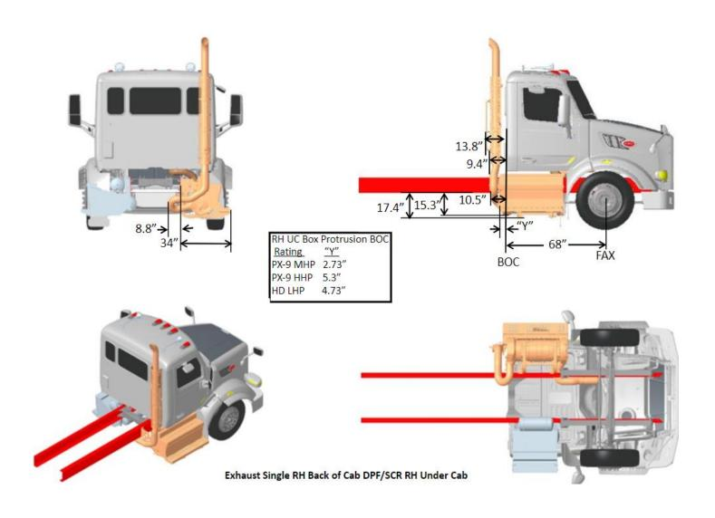
FIGURE 3-45. Exhaust Single RH Back of Cab DPF/SCR RH Under Cab
