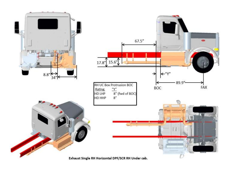
FIGURE 3-35. Exhaust Single RH Horizontal DPF/SCR RH Under Cab
