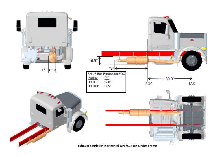
FIGURE 3-36. Exhaust Single RH Horizontal DPF/SCR Under Frame
