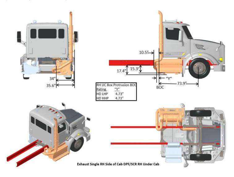
FIGURE 3-60. Exhaust Single RH Side of Cab DPF/SCR RH Under Cab
