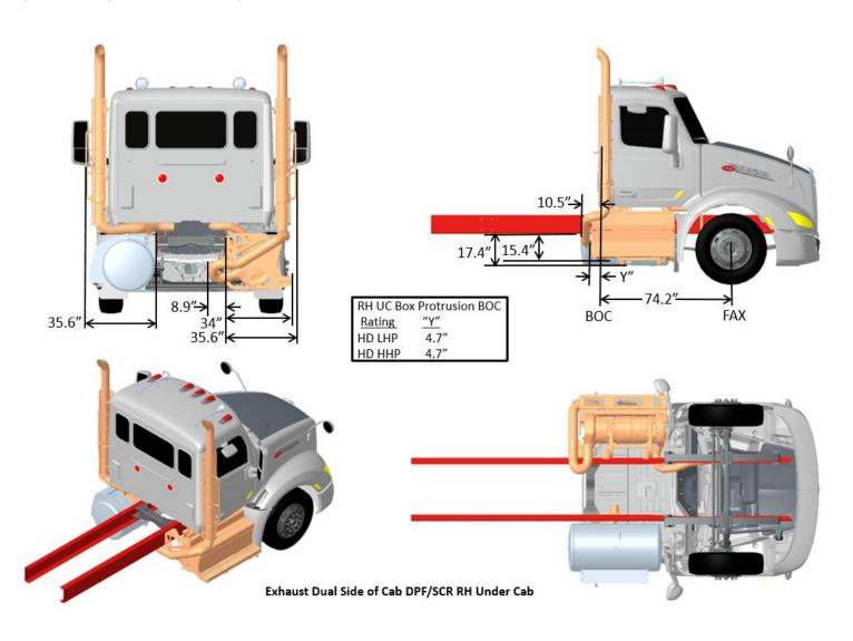
FIGURE 3-84. Exhaust Dual Side of Cab RH DPF/SCR RH Under Cab
