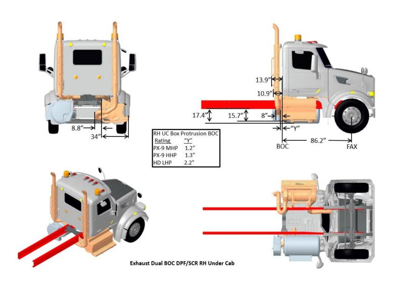
FIGURE 3-57. Exhaust Dual BOC DPF/SCR RH Under Cab
