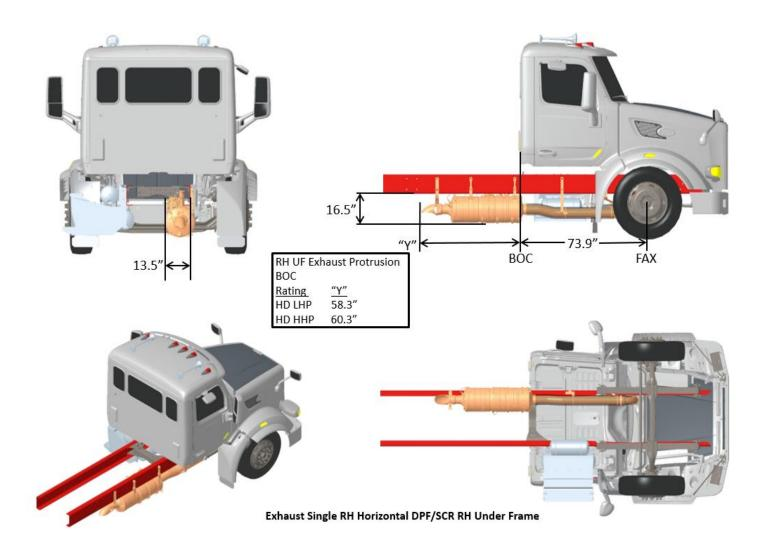
FIGURE 3-62. Exhaust Single RH Horizontal DPF/SCR RH Under Frame
