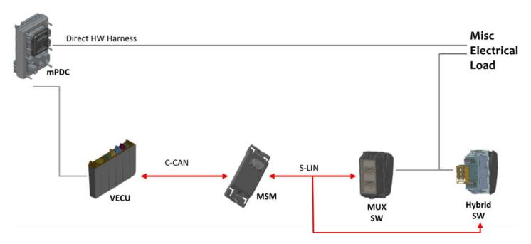
Multiplexing = shorter wire bundles, improved diagnostics, and greater driver feedback. Safety critical switches use hybrid switch with hardwire for redundancy. The switches are less expensive with fewer wires behind the dash and on the chassis. The switches are self-diagnosable to improve troubleshooting with DAVIE.
