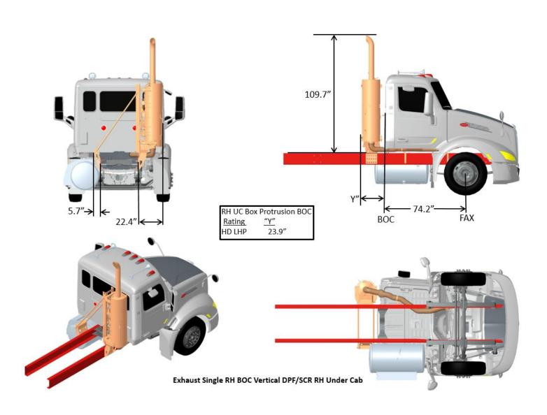
FIGURE 3-86. Exhaust Single RH BOC Vertical DPF/SCR
