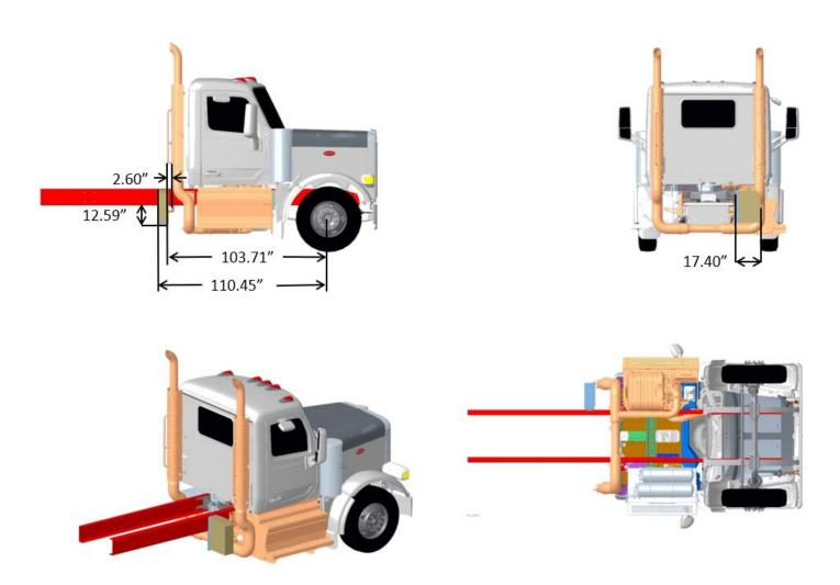
FIGURE 3-91. Exhaust Dual Back of Cab DPF/SCR RH Under Cab (functioning), Compact Twin
