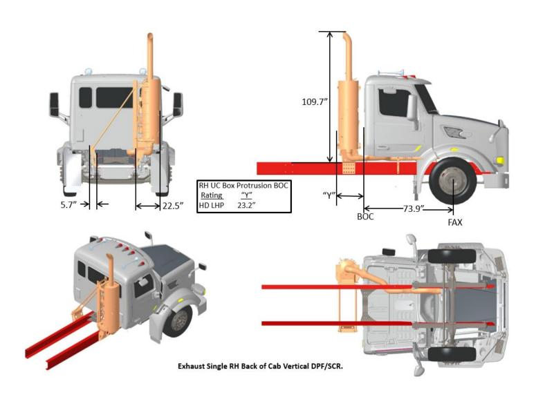
FIGURE 3-64. Exhaust Single RH BOC Vertical DPF/SCR
