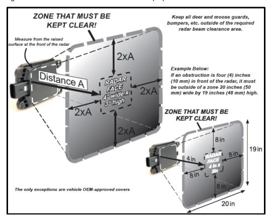
FIGURE 2-5: Fusion 2.0 Radar Clearance
