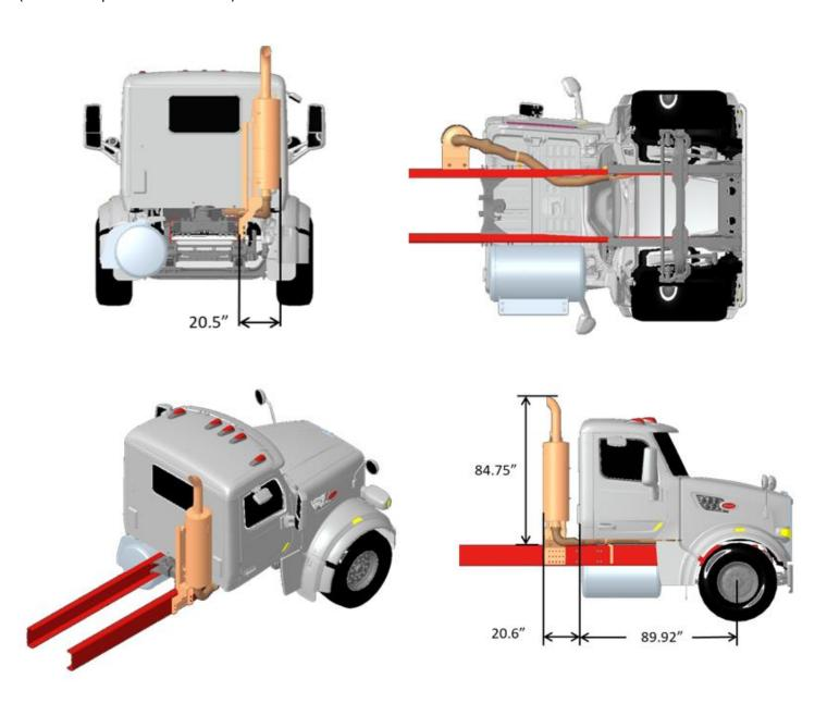
FIGURE 11-23: Model 567-121 SFFA RH Frame Mounted (Vertical) Exhaust
