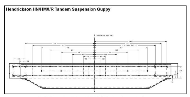
FIGURE 3-24. Hendrickson HN/HMX/R Tandem Suspension Guppy
