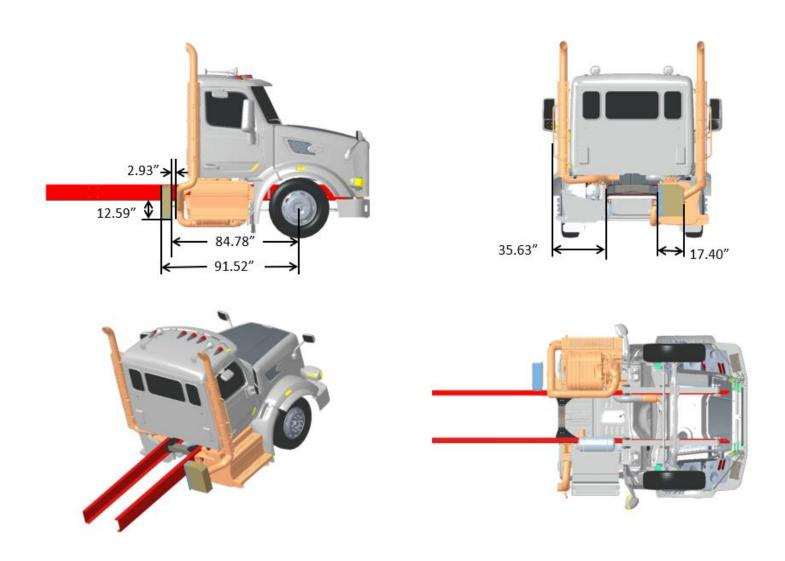
FIGURE 3-110. Exhaust Dual Side of Cab, LH SOC Stack Aesthetic, DPF/SCR RH Under Cab, Compact Twin
