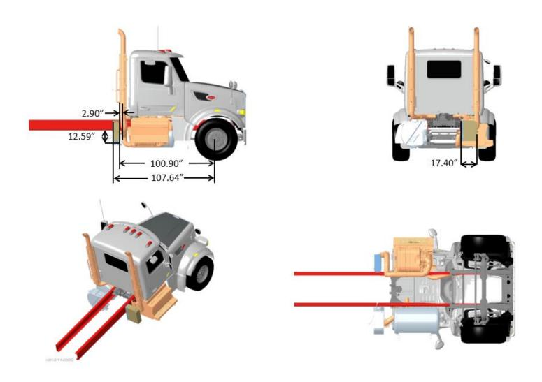
FIGURE 3-115. Exhaust Dual Back of Cab, LH BOC Stack Aesthetic Only, DPF/SCR RH Under Cab, Compact Twin
