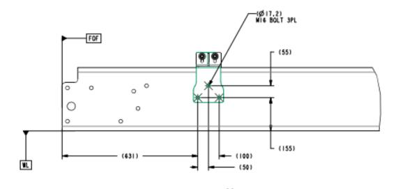
FIGURE 11-9: Fuel Filter Location for PB 579-124 (with Front Air Leaf Suspension)
