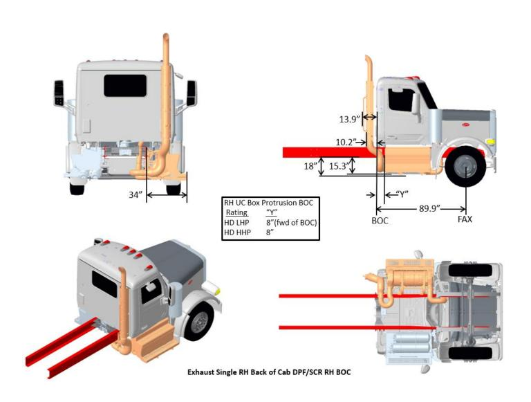
FIGURE 3-33. Exhaust Single RH Back of Cab DPF/SCR RH Under Cab
