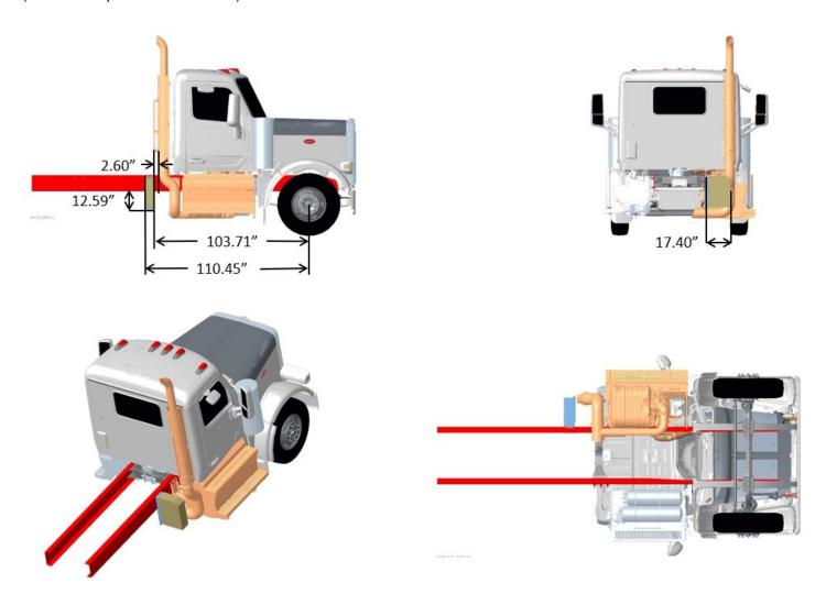
FIGURE 3-87. Exhaust Single RH Back of Cab DPF/SCR RH Under Cab, Compact Twin
