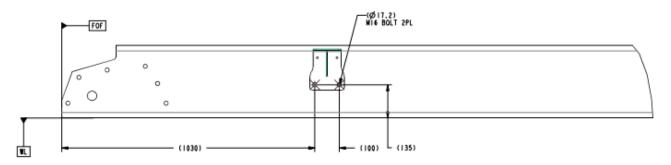
FIGURE 11-10: Fuel Filter Location for PB 567-121 SFFA
