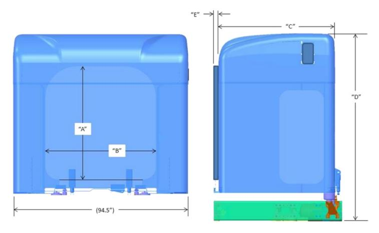
FIGURE 3-13. Sleeper Dimensions - Front & LH View
