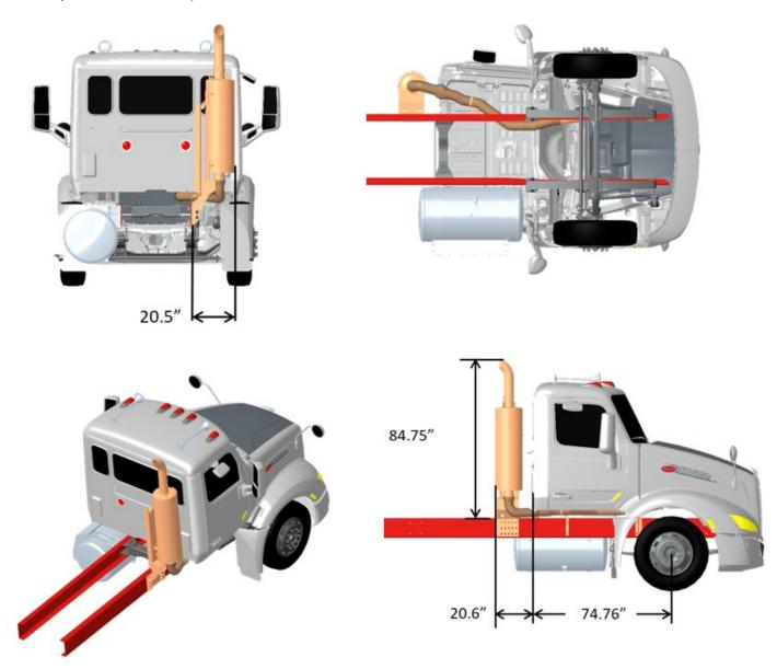
FIGURE 11-20: Model 579-124 RH Side of Cab Exhaust
