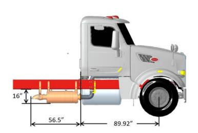
FIGURE 11-21: Model 567-121 SFFA RH Horizontal Underframe Exhaust
