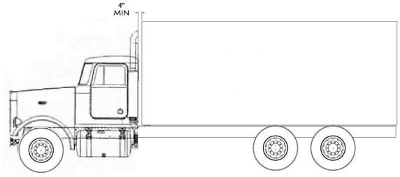
FIGURE 4-2. Minimum Back of Cab Clearance
