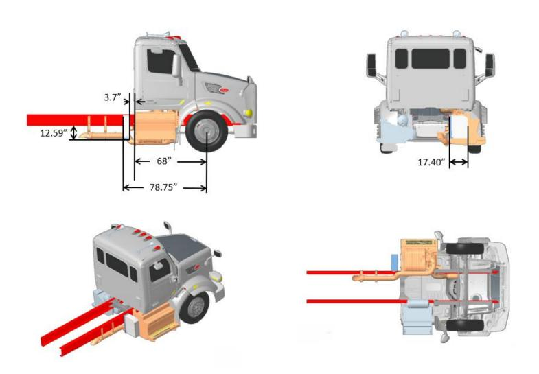
FIGURE 3-99. Exhaust Single RH Horizontal DPF/SCR RH Under Cab, Compact Twin
