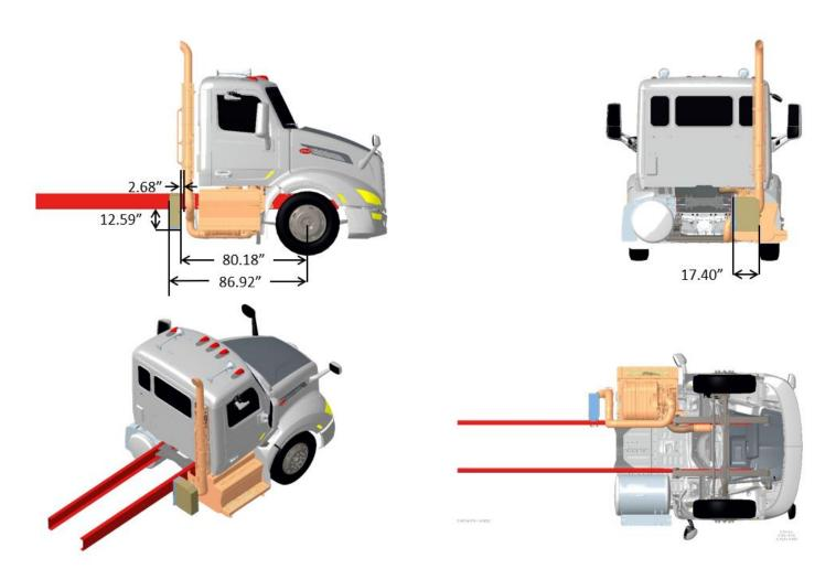
FIGURE 3-117. Exhaust Single RH Back of Cab DPF/SCR RH Under Cab, Compact Twin
