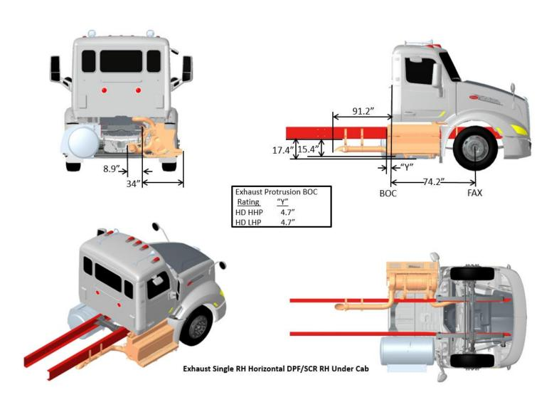
FIGURE 3-82. Exhaust Single RH Horizontal DPF/SCR RH Under Cab
