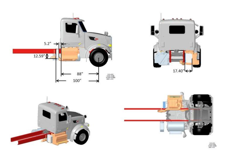
FIGURE 3-114. Exhaust Single RH Horizontal DPF/SCR RH Under Cab, Compact Twin
