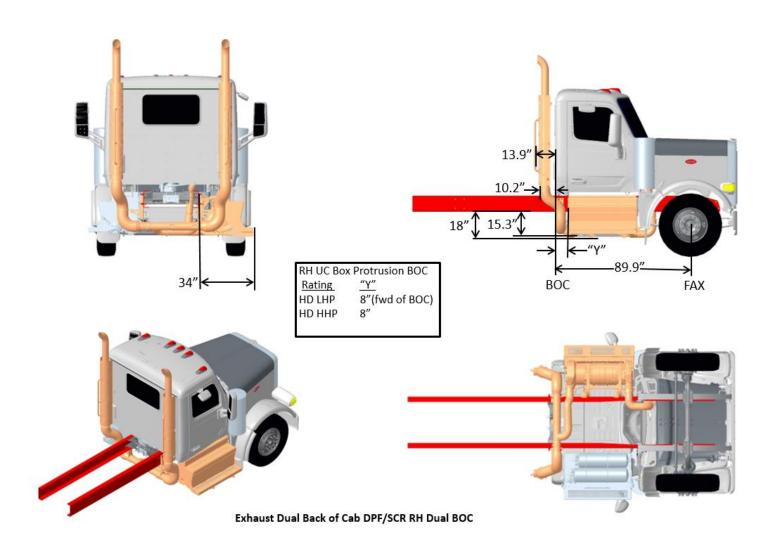
FIGURE 3-38. Exhaust Dual Back of Cab DPF/SCR RH Under Cab (functioning)
