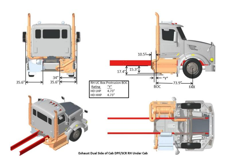
FIGURE 3-63. Exhaust Dual SOC DPF/SCR RH Under Cab
