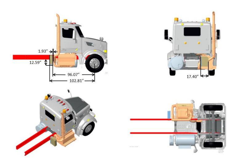
FIGURE 3-103. Exhaust Single RH Side of Cab DPF/SCR RH Under Cab, Compact Twin
