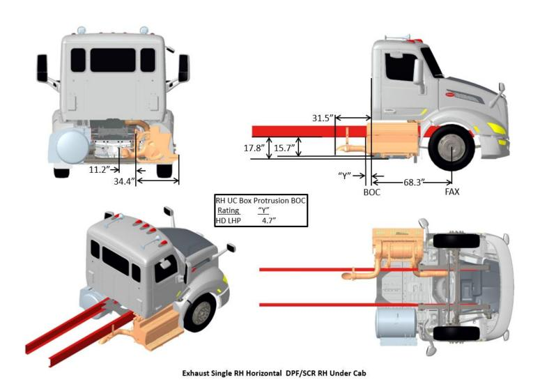
FIGURE 3-75. Exhaust Single RH Horizontal DPF/SCR RH Under Cab
