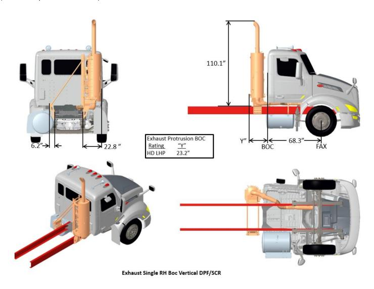
FIGURE 3-79. Exhaust Single RH BOC Vertical DPF/SCR
