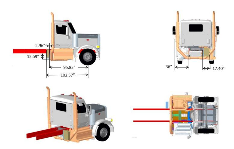
FIGURE 3-90. Exhaust Dual Side of Cab DPF/SCR RH Under Cab (functioning), Compact Twin
