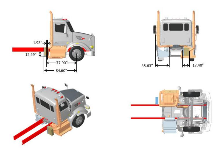
FIGURE 3-101. Exhaust Dual Side of Cab, LH SOC stack aesthetic only, RH Under Cab DPF/SCR, Compact Twin
