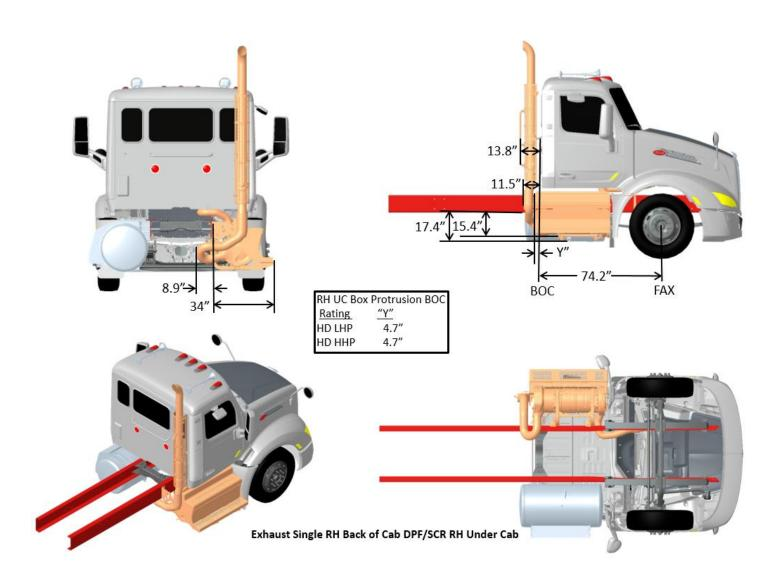
FIGURE 3-80. Exhaust Single RH Back of Cab DPF/SCR RH Under Cab
