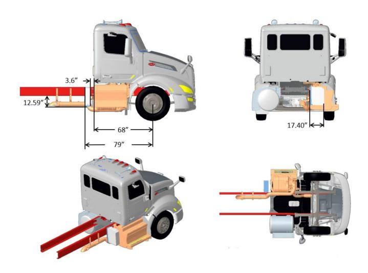
FIGURE 3-119. Exhaust Single RH Horizontal DPF/SCR RH Under Cab, Compact Twin
