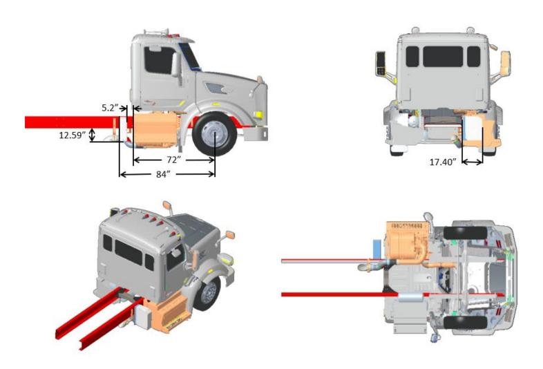
FIGURE 3-109. Exhaust Single RH Horizontal DPF/SCR RH Under Cab, Compact Twin
