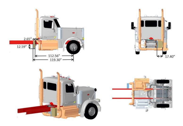
FIGURE 3-96. Exhaust Dual Back of Cab DPF/SCR RH Under Cab (Functioning), Compact Twin
