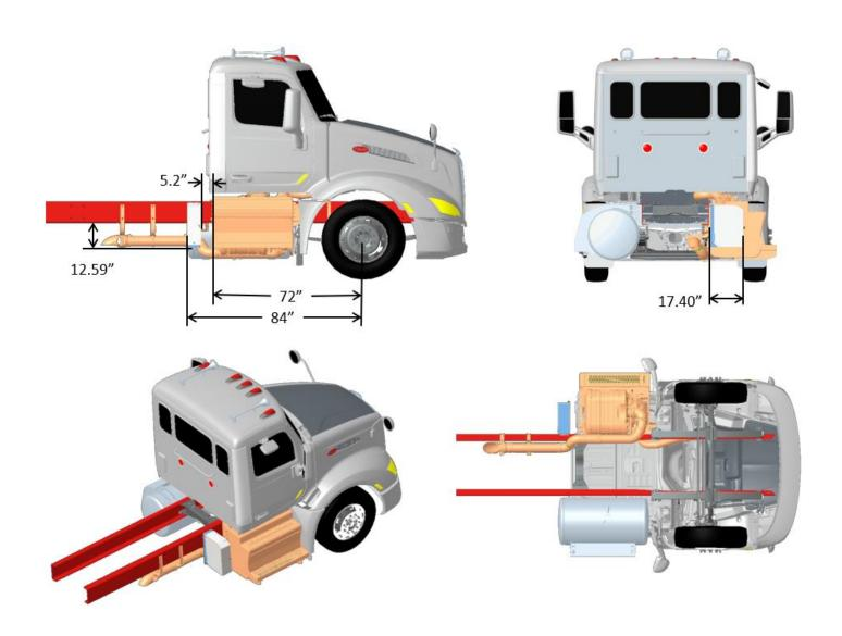
FIGURE 3-124. Exhaust Single RH Horizontal DPF/SCR RH Under Cab, Compact Twin
