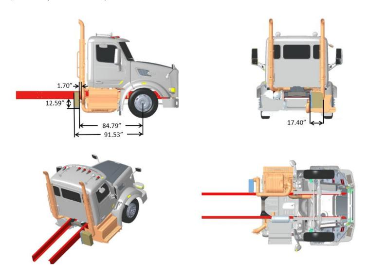
FIGURE 3-111. Exhaust Dual Back of Cab, LH BOC Stack Aesthetic, DPF/SCR RH Under Cab, Compact Twin
