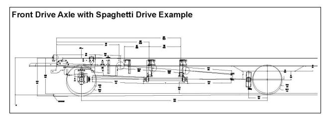
FIGURE 3-16. Front Drive Axle with Spaghetti Drive Example
