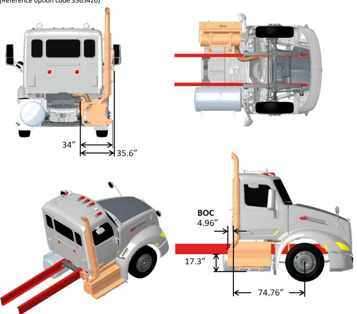
FIGURE 11-19: Model 579-124 RH Side of Cab Exhaust
