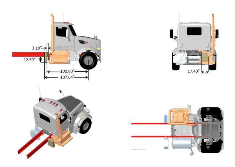
FIGURE 3-113. Exhaust Single RH Side of Cab DPF/SCR RH Under Cab, Compact Twin
