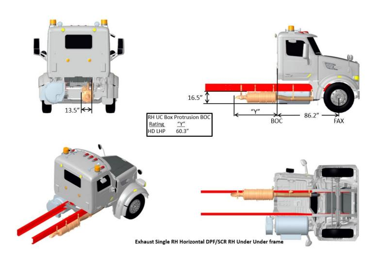
FIGURE 3-55. Exhaust Single RH Horizontal DPF/SCR RH Under Frame
