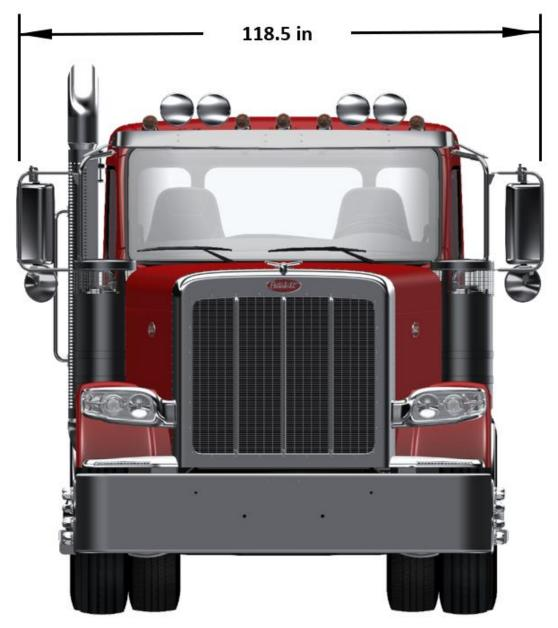
FIGURE 3-3. Model 589-121 Front View – Overall Dimensions
