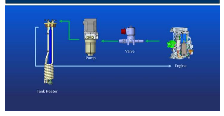
FIGURE 9-1. DEF System Schematic
