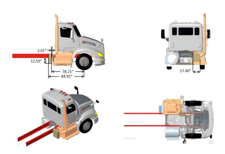
FIGURE 3-118. Exhaust Single RH Side of Cab DPF/SCR RH Under Cab, Compact Twin
