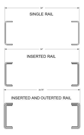
FIGURE 3-14. Frame Rail Configurations
