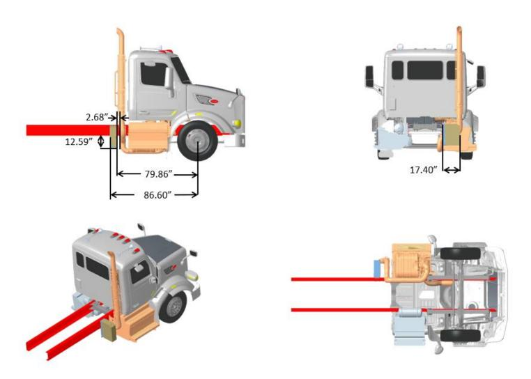
FIGURE 3-97. Exhaust Single RH Back of Cab DPF/SCR RH Under Cab, Compact Twin
