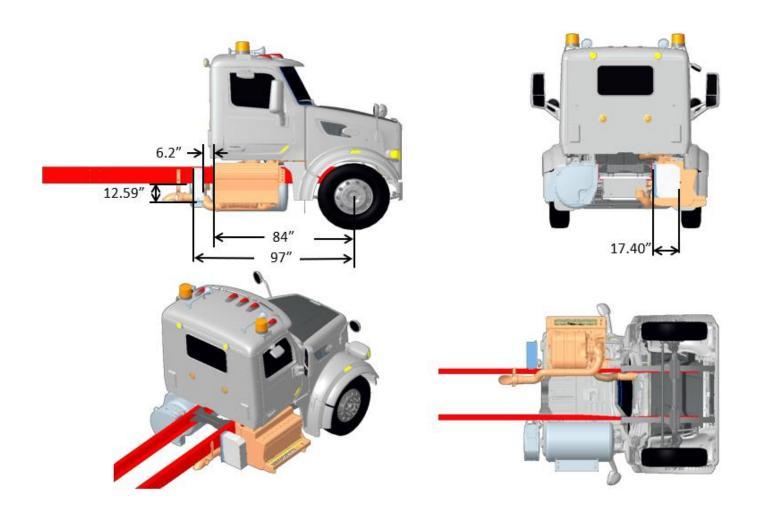
FIGURE 3-104. Exhaust Single RH Horizontal DPF/SCR RH Under Cab, Compact Twin
