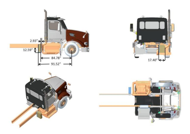
FIGURE 3-108. Exhaust Single RH Side of Cab DPF/SCR RH Under Cab, Compact Twin
