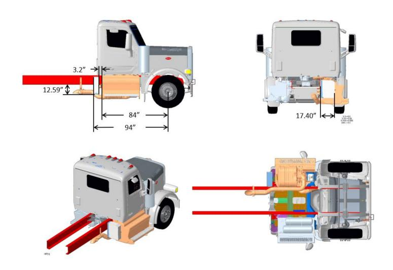
FIGURE 3-89. Exhaust Single RH Horizontal DPF/SCR RH Under Cab, Compact Twin
