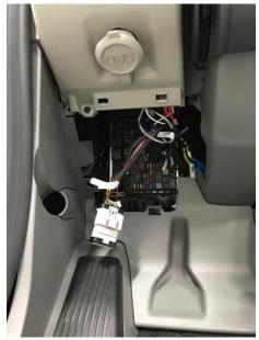
RP1226 Connector Inside the Cab (See "Section 7 Electrical" For More Locations)
