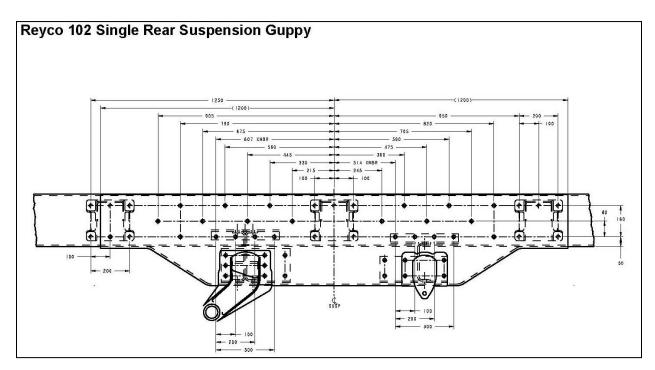
FIGURE 3-27. Reyco 102 Single Drive Suspension Guppy
