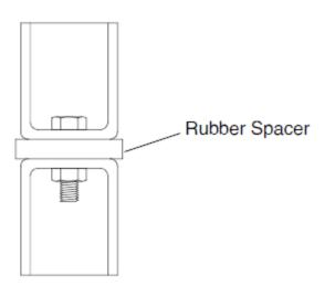
FIGURE 4-5. Mounting Brackets
