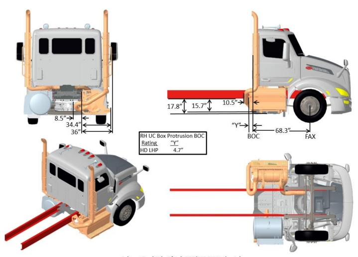
Exhaust Dual Side Of Cab DPF/SCR RH Under Cab
