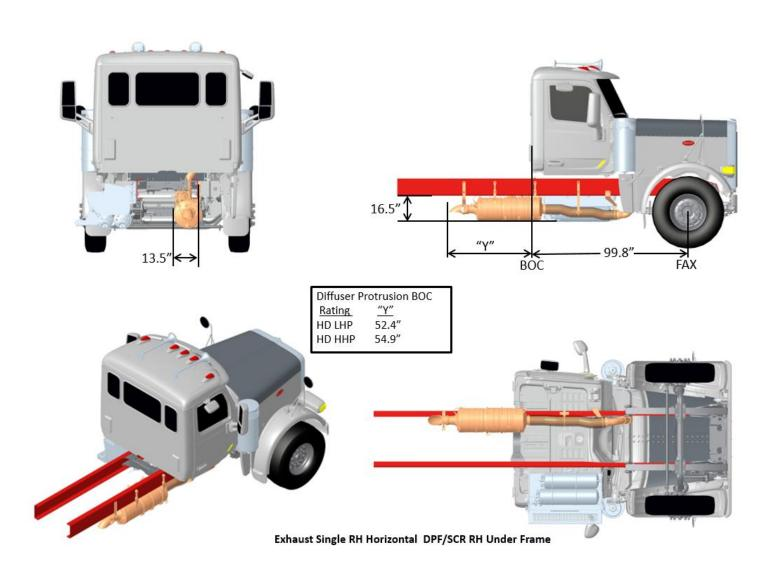
FIGURE 3-42. Exhaust Single RH Horizontal DPF/SCR Under Frame
