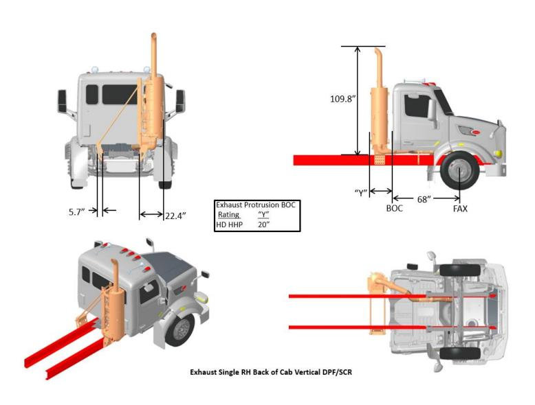
FIGURE 3-51. Exhaust Single RH BOC Vertical DPF/SCR
