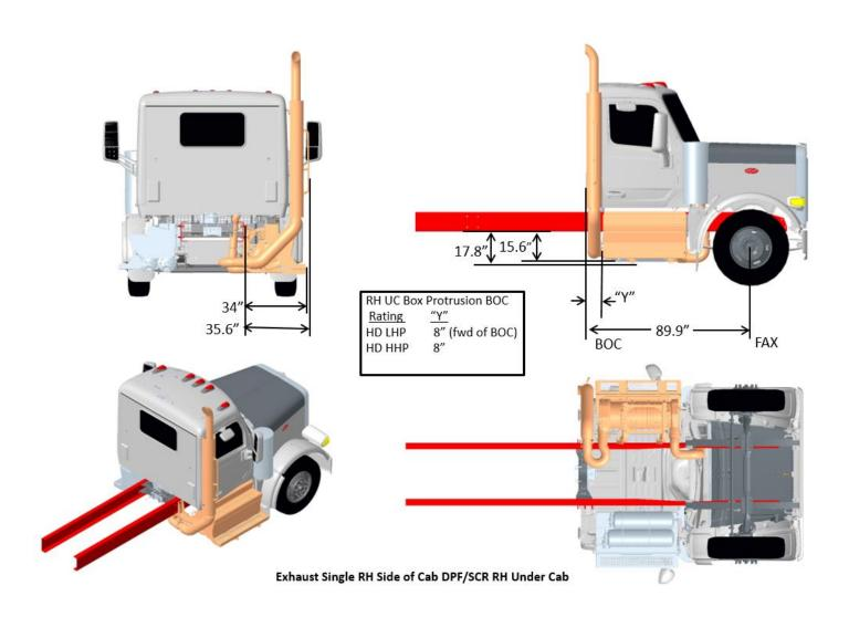
FIGURE 3-34. Exhaust Single RH Side of Cab DPF/SCR RH Under Cab
