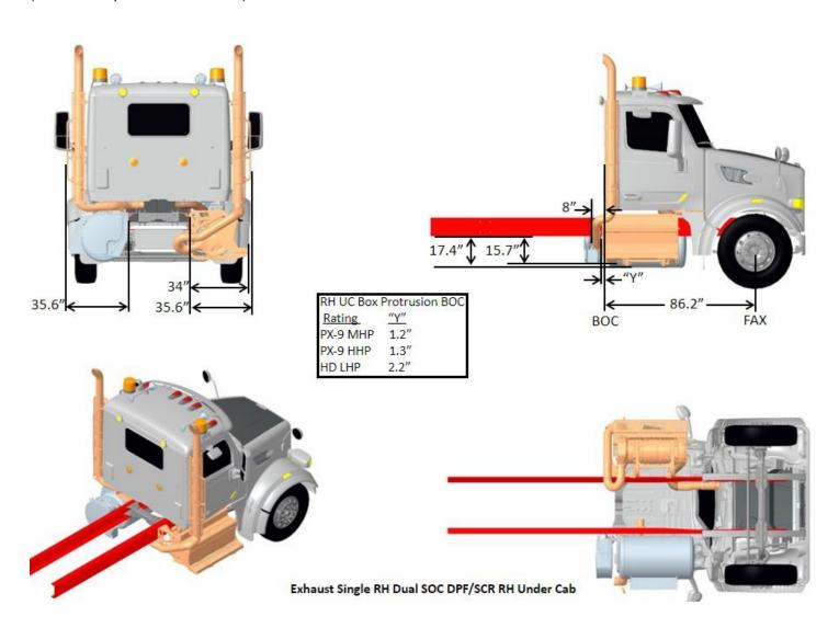
FIGURE 3-55. Exhaust Dual SOC DPF/SCR RH Under Cab
