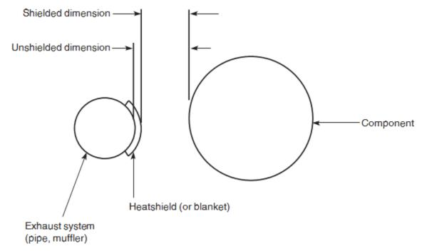
FIGURE 10-5. Definition of measurements.
