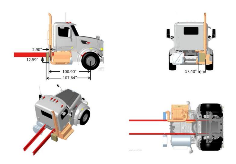
FIGURE 3-112. Exhaust Single RH Back of Cab DPF/SCR RH Under Cab, Compact Twin
