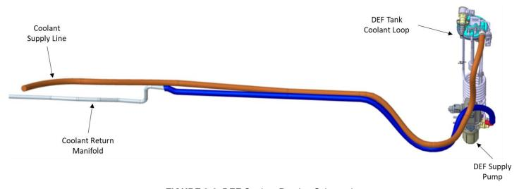
FIGURE 9-2. DEF Coolant Routing Schematic
