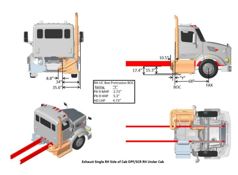
FIGURE 3-46. Exhaust Single RH Side of Cab DPF/SCR RH Under Cab
