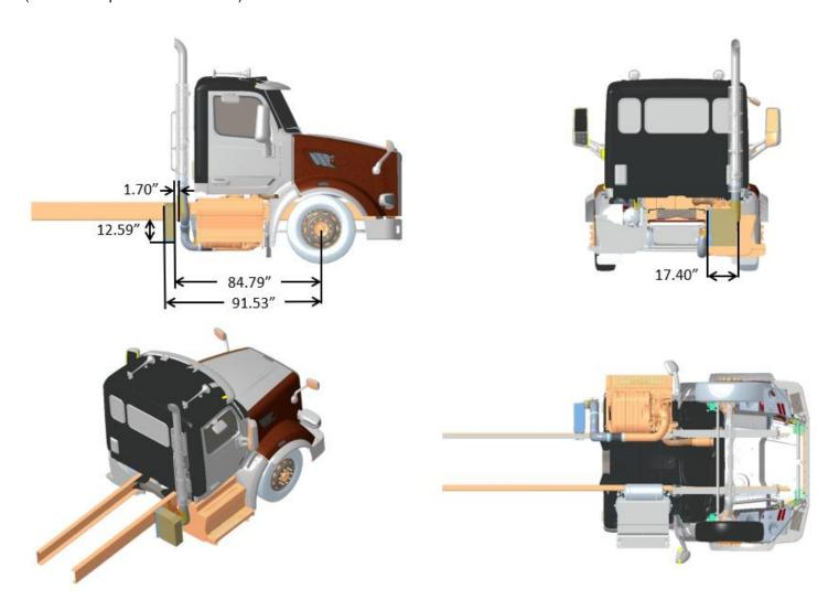
FIGURE 3-107. Exhaust Single RH Back of Cab DPF/SCR RH Under Cab, Compact Twin
