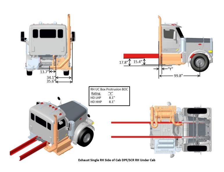
FIGURE 3-40. Exhaust Single RH Side of Cab DPF/SCR RH Under Cab
