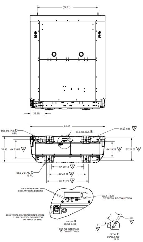
FIGURE 11-13: Back of Cab System
