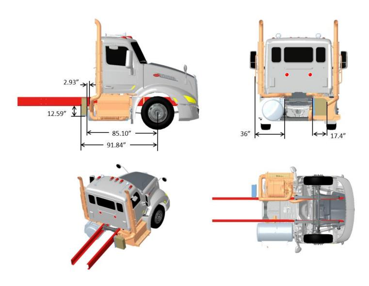
FIGURE 3-126. Exhaust Dual Side of Cab, LH SOC Stack Aesthetic Only, DPF/SCR RH Under Cab, Compact Twin
