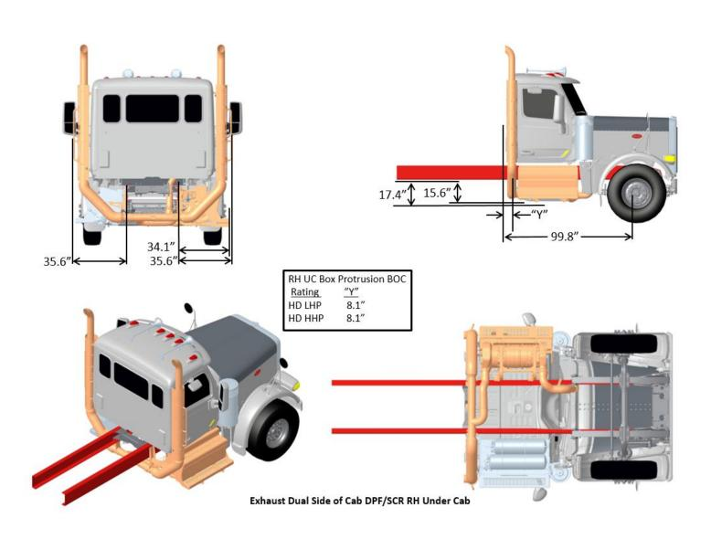
FIGURE 3-43. Exhaust Dual Side of Cab DPF/SCR RH Under Cab (functioning)
