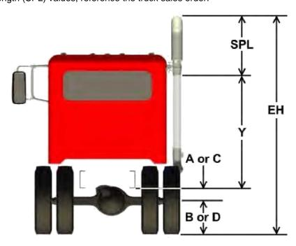
FIGURE 3-28. Exhaust Height Calculations
