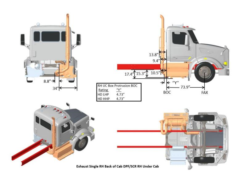
FIGURE 3-59. Exhaust Single RH Back of Cab DPF/SCR RH Under Cab
