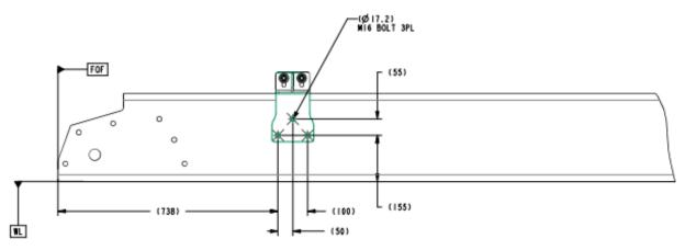
FIGURE 11-12: Fuel Filter Location for PB 567-121 SBFA (with Front Air Leaf Suspension)
