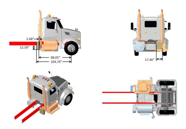
FIGURE 3-106. Exhaust Dual Back of Cab, LH BOC Aesthetic Only, DPF/SCR RH Under Cab, Compact Twin
