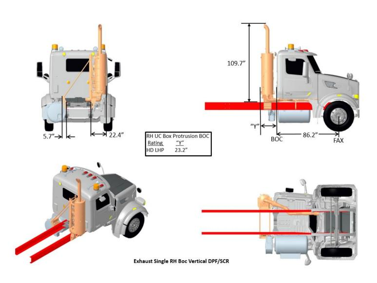
FIGURE 3-58. Exhaust Single RH BOC Vertical DPF/SCR
