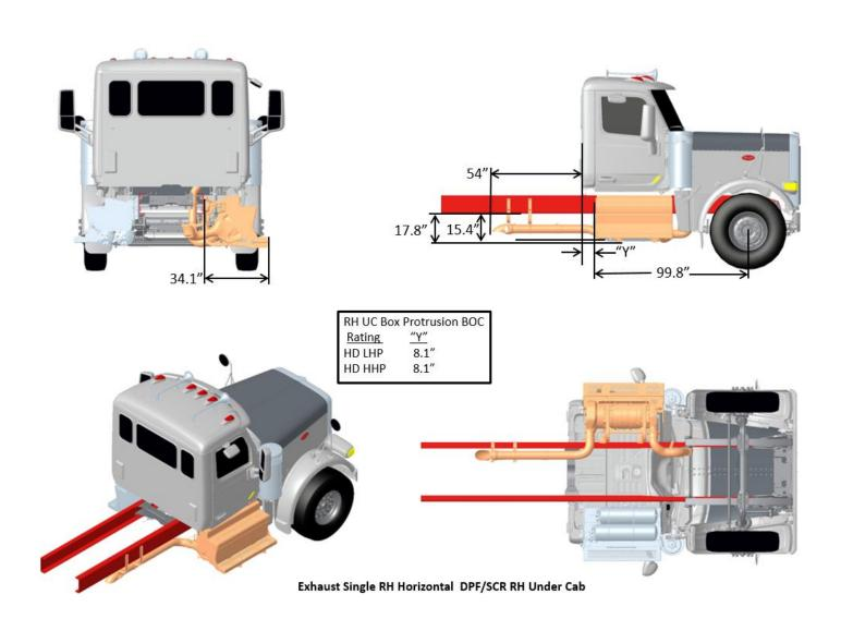
FIGURE 3-41. Exhaust Single RH Horizontal DPF/SCR RH Under Cab
