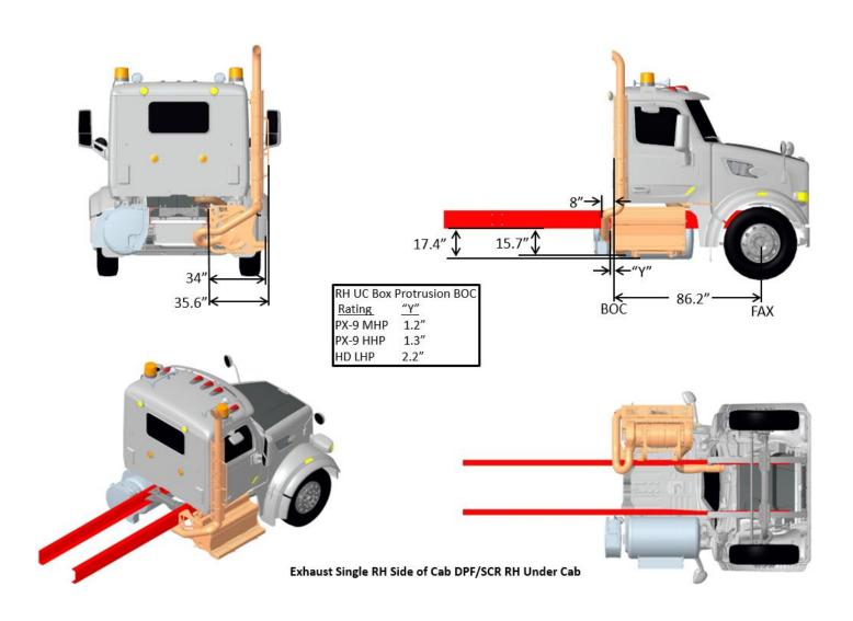
FIGURE 3-53. Exhaust Single RH Side of Cab DPF/SCR RH Under Cab
