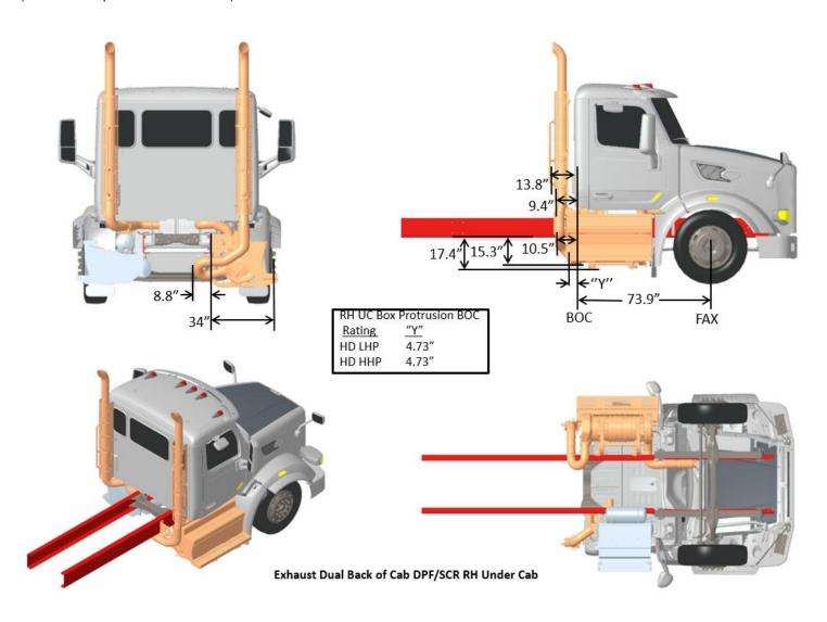
FIGURE 3-65. Exhaust Dual Back of Cab DPF/SCR RH Under Cab
