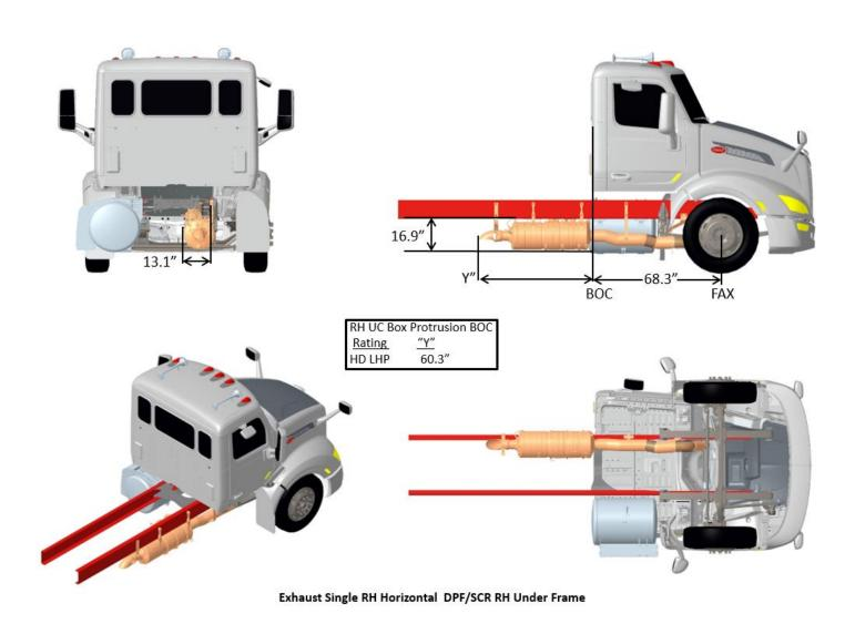
FIGURE 3-76. Exhaust Single RH Horizontal DPF/SCR RH Under Frame
