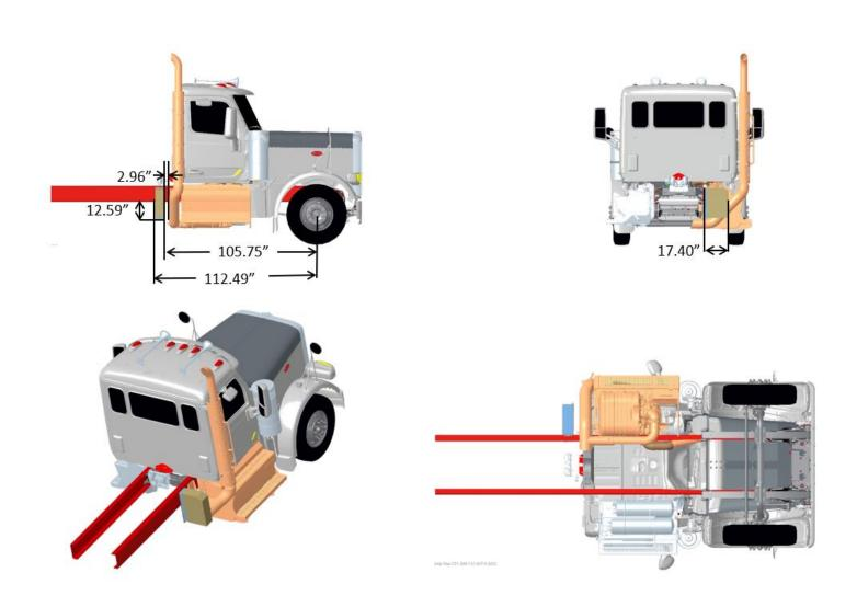
FIGURE 3-93. Exhaust Single RH Side of Cab DPF/SCR RH Under Cab, Compact Twin
