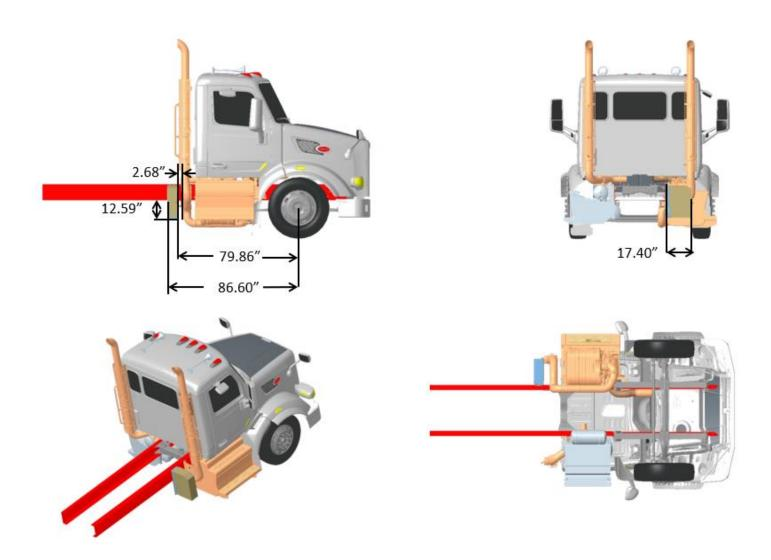
FIGURE 3-100. Exhaust Dual Back of Cab, LH BOC stack aesthetic only, RH Under Cab DPF/SCR, Compact Twin
