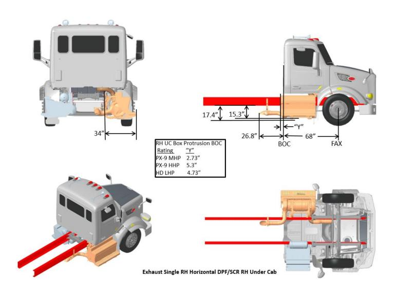
FIGURE 3-47. Exhaust Single RH Horizontal DPF/SCR RH Under Cab
