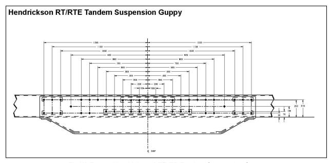
FIGURE 3-26. Hendrickson RT/RTE Tandem Suspension Guppy
