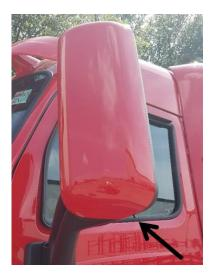
FIGURE 2-3: Aerodynamic Mirror OAT Sensor Location
