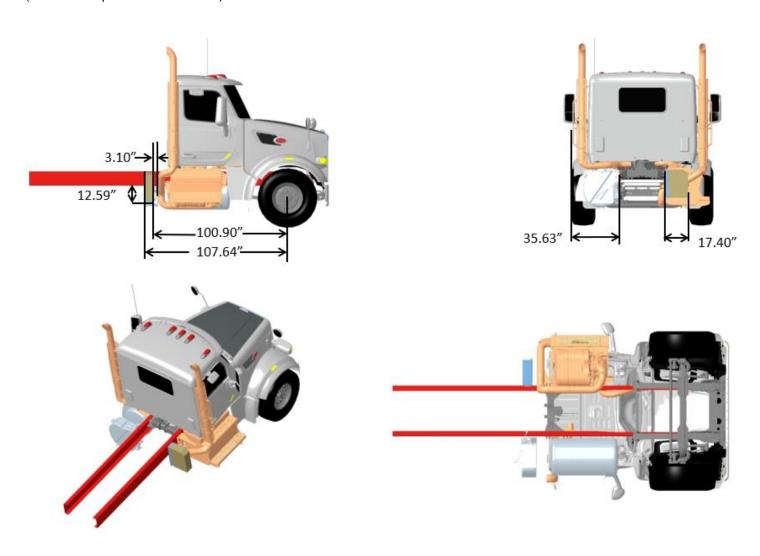
FIGURE 3-116. Exhaust Dual Side of Cab, LH SOC Stack Aesthetic Only, DPF/SCR RH Under Cab, Compact Twin
