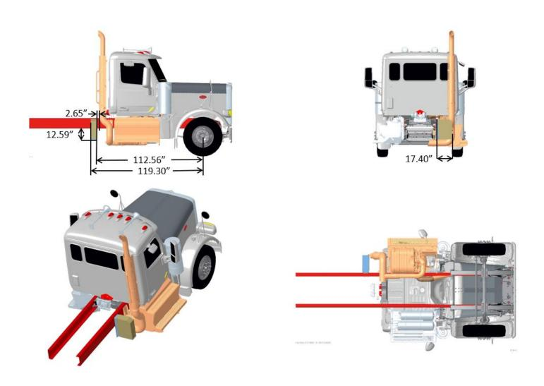
FIGURE 3-92. Exhaust Single RH Back of Cab DPF/SCR RH Under Cab, Compact Twin
