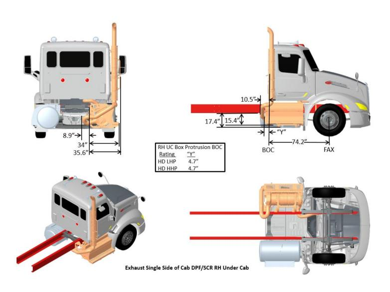
FIGURE 3-81. Exhaust Single RH Side of Cab DPF/SCR RH Under Cab
